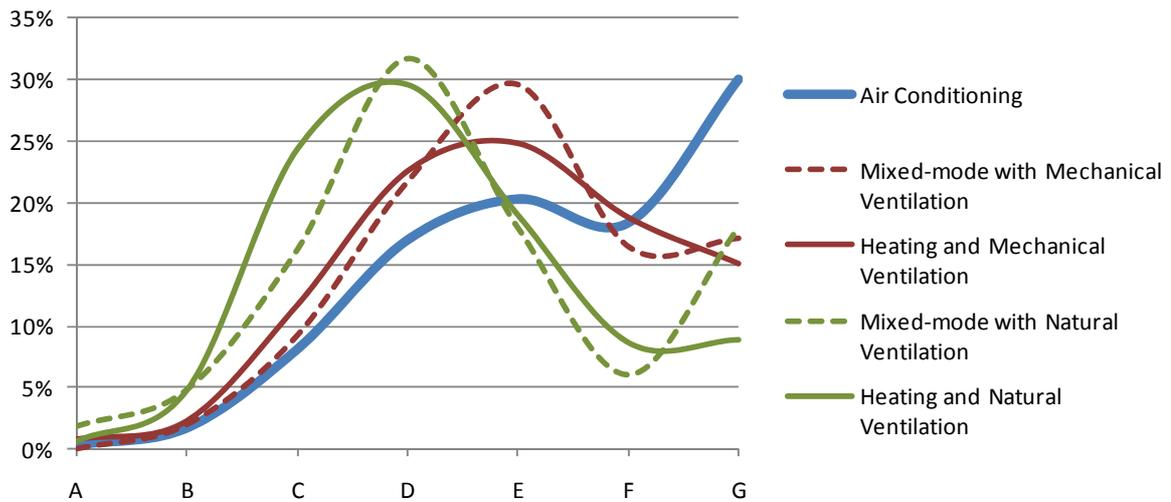
**Fig C.3** Distribution of ratings by HVAC type for 2,311 'offices' from the 2010 DEC database
